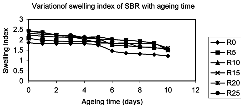
FIGURE 14 Variation of swelling index with ageing time of SBR vulcanizates with different resin contents.
